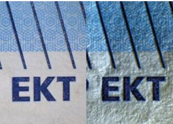
€20 banknote: Ring light illumination / horizontal illumination
